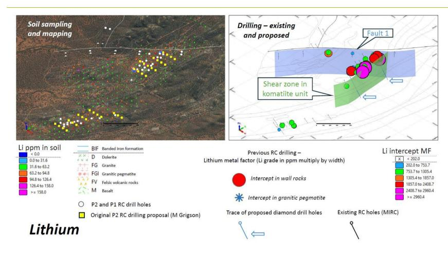
Figure 1: The two proposed deep diamond holes to test for spodumene bearing pegmatites
